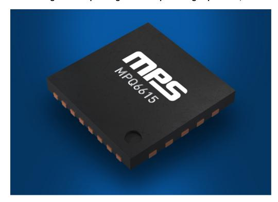
The MP6615 from Monolithic Power Systems is an integrated H-bridge dc motor driver which implements a full bridge made up of four N-channel power MOSFETs. The motor driver also integrates pre-drivers, gate driver power supplies, and bidirectional current-sense amplifiers, enabling designers to reduce component count, simplify their board layout and save space.
