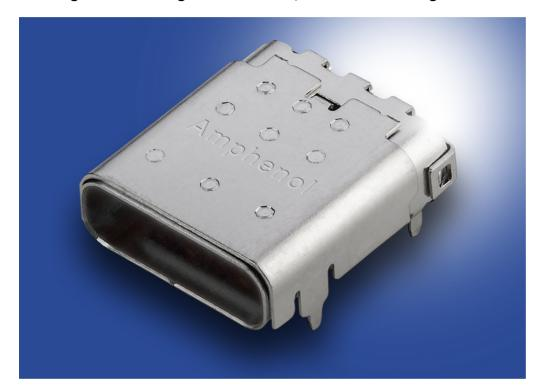
USB Type-C connectors from Amphenol Communications Solutions support various USB protocols, such as USB 2.0, USB 3.0, USB 3.1, and USB 3.2, to provide features including a 10 Gbits/s data rate, and 5 A/20 V power capability.
